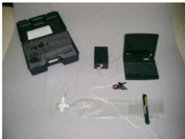
Fig. 1. In the back left is the carry case. To the back right is the pressure transducer and computer. In the front is shown the mouth piece with inspiratory and expiratory spring loaded valves.
